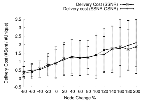
Figure 5. RM dataset. Message delivery cost vs target percentage modification of each message sender's social network. As we obfuscate the sender's social network by adding links, the delivery cost increases.
