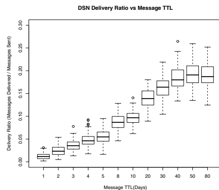
(b) Delivery ratio compared to message TTL, when the DSN is passed at each hop.
